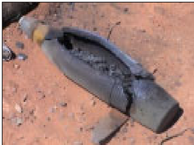
Post "AUSZIPPER" firing, 5"/54 Naval gun shell.
