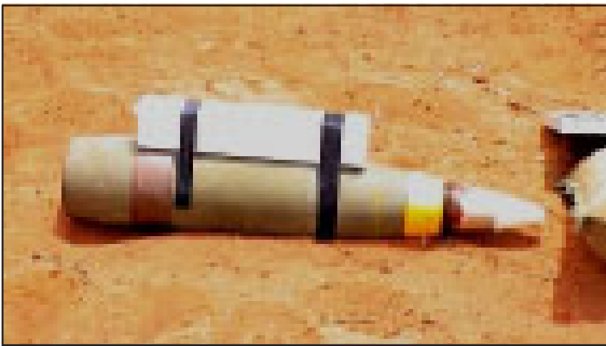
5"/54 Naval gun shell with "AUSZIPPER" set up for EOD
