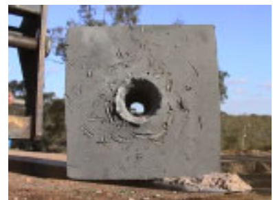
CDS 150 (250mm +) penetration in mild steel block
