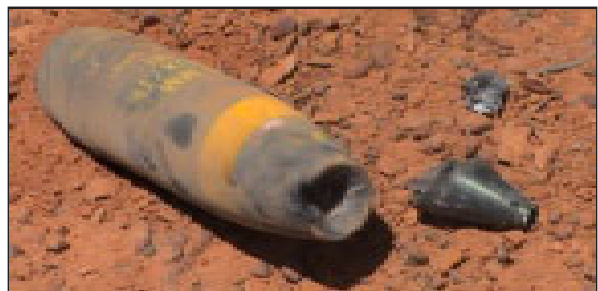
Post "AUSPLASTIC" firing, 105mm Howitzer shell fuze removed.
